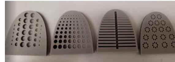
**Figure 3.** 3D printed breast inserts after the curing process. Printed using a photopolymer resin (Formlabs Inc Rigid resin).
