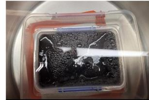
**Figure 2.** Gelatin breast phantom using graphite powder. The surface bubbles are a result of the vacuum chamber.
