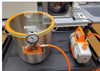
**Figure 1.** Using a vacuum chamber to extract air bubbles during the breast phantom creation process. Air bubbles could create unwanted artifacts if present during phantom creation.
